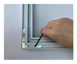
**3.** Assemble all the frame, then securely screw each junction using the Allen key.
