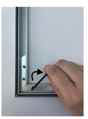
**4.** Assemble all the frame, then securely screw each junction using the Allen key.
