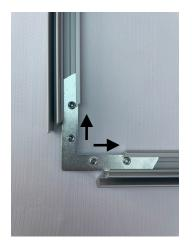
**3.** Insert one connectors at each corner, by sliding it into the groove of the extrusion.
