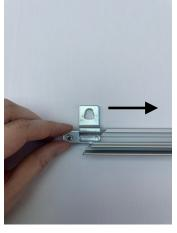
2. Insert and slide the mounting bracket(s) on the extrusions so that they will be evenly distributed to secure the frame onto the wall.
