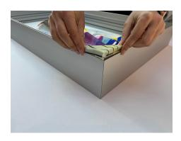
1. Take one corner of the fabric print and insert the silicone edge trim into the slot of the frame. Put this way each corner of the fabric print in the frame.
