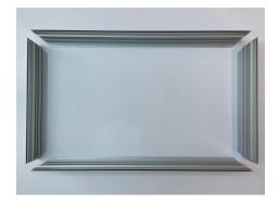
**1.** Position flat on a table the four extrusions of the frame's sides in order to form the frame.
